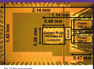
Fig. 2 Chip micrograph
