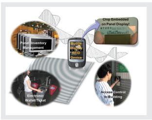
As shown in Fig. 1, the smart phone with an embedded LTPS TFT RFID tag turns into a mobile NFC device. It can be used for electronic ticketing and building access control. Moreover, the mobile NFC device can be further extended to include the function of electronic wallet to manage daily expense.
