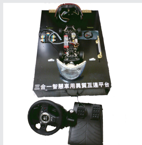
圖二 Fig.2 FlexRay / CAN / LIN之異質互連平台 FlexRay/CAN/LIN 3-to-1 Heterogeneous interconnection platform design
