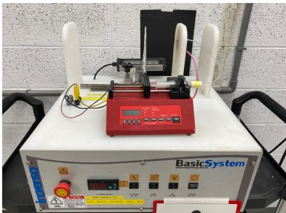
**Figure 4.** Image of Electrospinner Creating Carbon-Based Polymer Nanofibers
