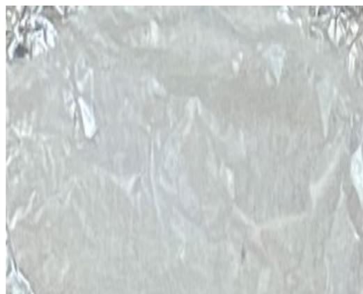
**Figure 5.** PAN-CuNP Nanofibers Coated on Aluminum Foil
