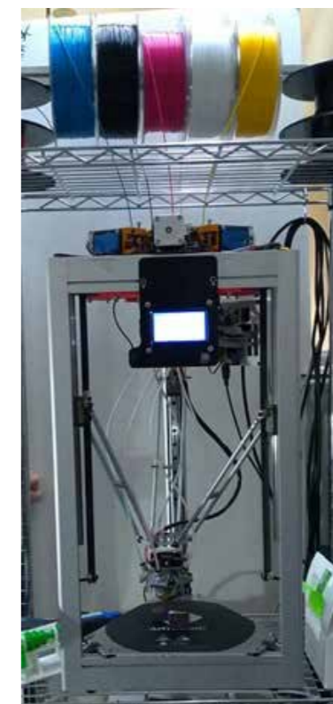
Fig.1 The multi-primary color FDM 3D printer
